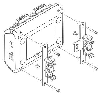
Figure 3-7. OM-DAQ-USB-2401 Rail Mounting
